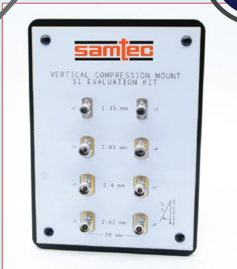
▲ Fig. 2 Samtec REF-228591 evaluation kit with multiple compression-mount connectors.
