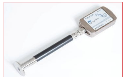
▲ Fig. 3 SPEAG DAK measurement system.
