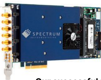
SERIES: M4i (17 models) TYPE: PCIe x8 with 8 to 16 bit SPEED: 180 MS/s to 5 GS/s CHANNELS: 1 to 4
