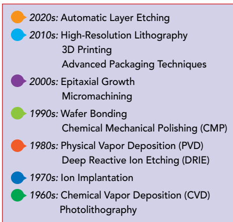
Fig. 2 Process techniques for high frequency component fabrication.
