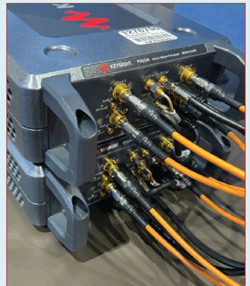
Fig. 1 Samtec Nitrowave™ cables in a test application using Keysight P502A USB VNAs.
